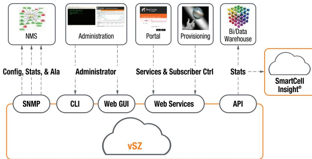
Figure 2: The built-in EMS in the vSZ-H provides user-friendly full-fledged FCAPS support and can be easily integrated with existing OSS/BSS systems.
